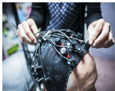
The fNIRS cap used to measure blood oxygen changes in the brain
